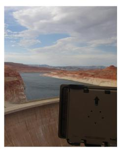
In this potential waterfront setup, a CC8A coordinates the efforts of two rotating cameras and two SpotterRF radars. Movement toward the dam in the low-alert zone and any movement in the high alert zone triggers an alert and cues one of the two rotating cameras to start recording video.
